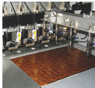
The MIL software can process image data from a flexible printed-circuit panel. Courtesy of Matrox Imaging.
